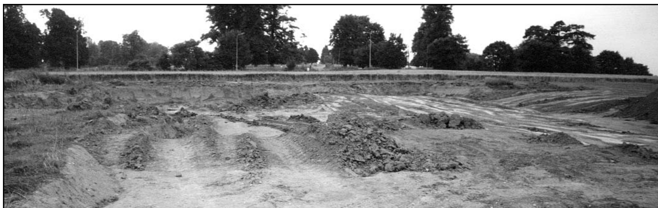
Figure 1. Loess exposed in a shallow brick pit at Ospringe, near Faversham. About 2 m of leached brickearth is worked to make distinctive orange bricks, while 2 m of unleached material is left in place.
